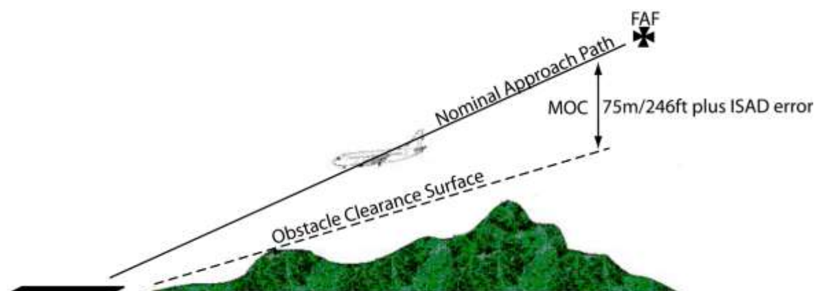
Figure 9.6: Baro-VNAV obstacle clearance for RNP APCH – LNAV
