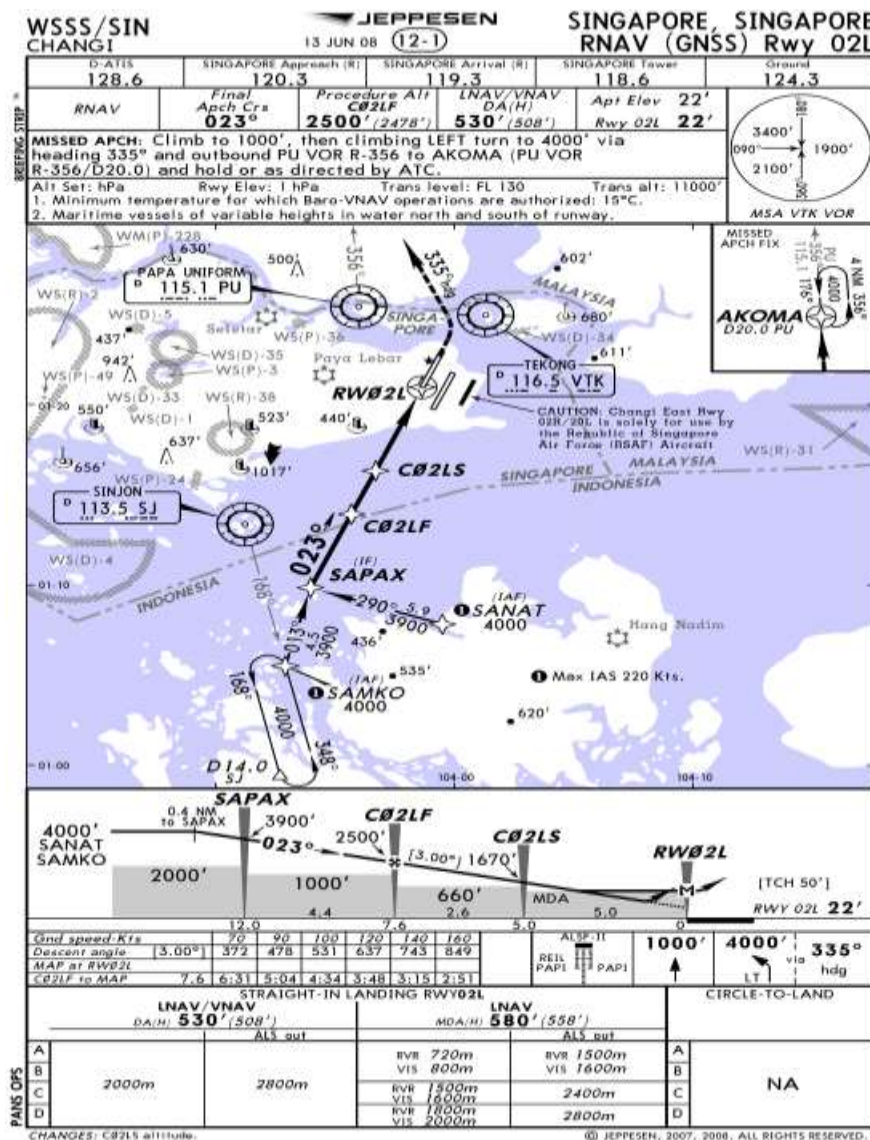
Figure 9.4 RNAV (GNSS) Approach Chart with LNAV and LNAV/VNAV Minima
