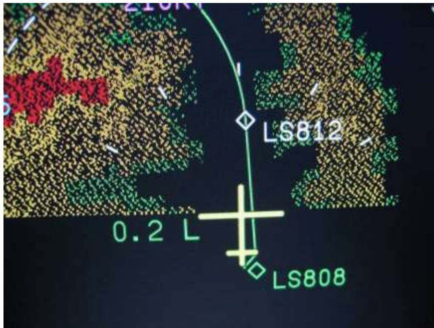
Fig 7.2: Example of cross-track deviation display in 1/10^{\text{th}} NM
