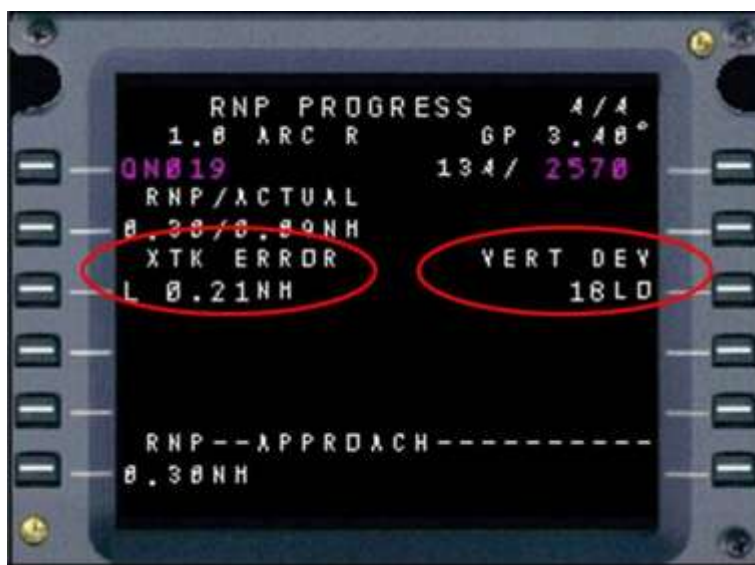
Figure 7.1: Cross-track and Vertical Deviations shown on Control and Display Unit
