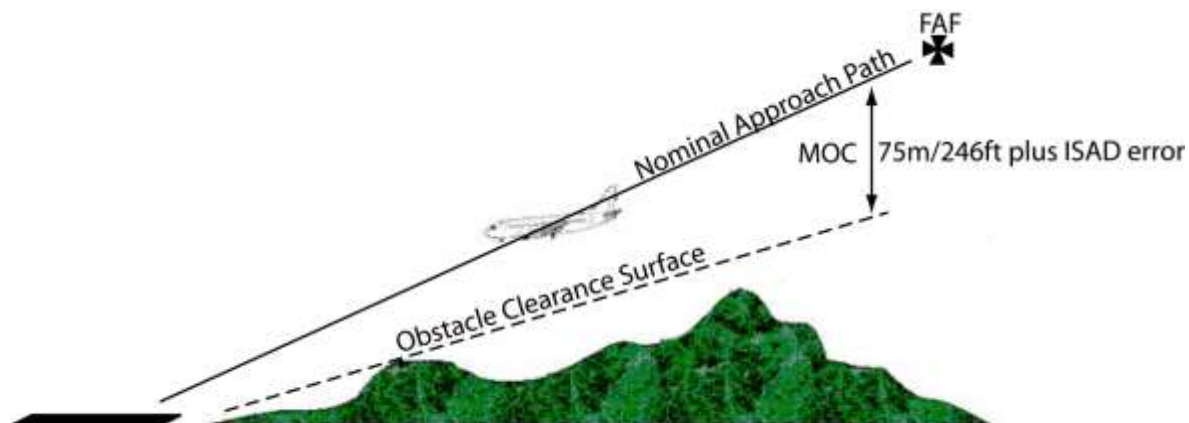
Figure 6.4: RNP APCH (LNAV/VNAV) Final Segment Obstacle Clearance
