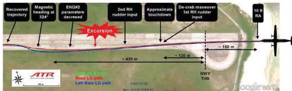
Figure 4 : Reconstructed landing path based on QAR read out
