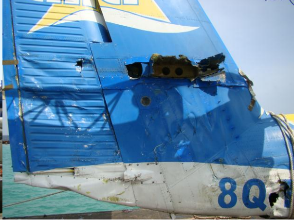
Damage during salvage operation
