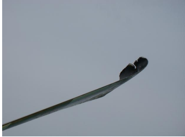
LH propeller blade damage
