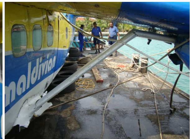
LH wing strut damaged
