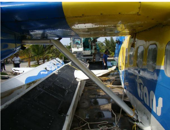
RH wing strut damaged
