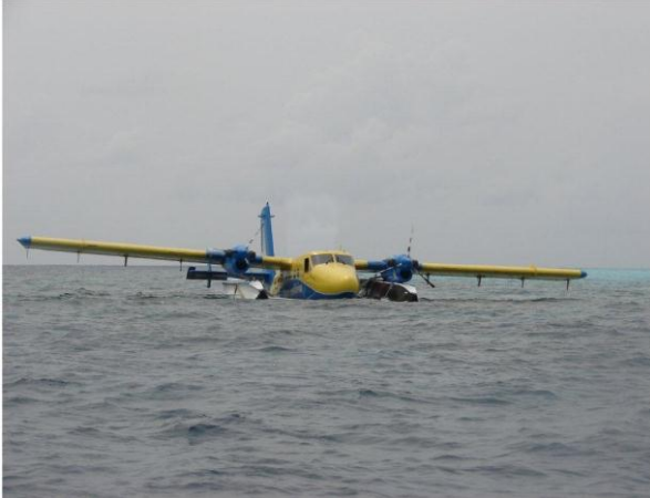
Both floats almost detached from aircraft and twisted
