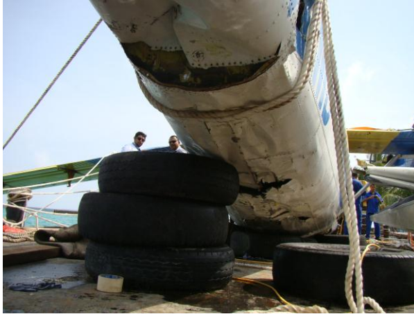
Secondary damage by current, reef and waves
