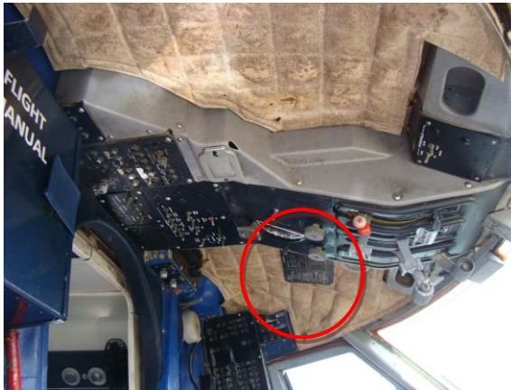
Flap selector shows zero flaps
