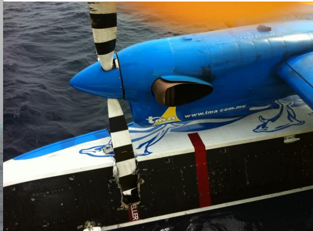
Propeller cut on right float
